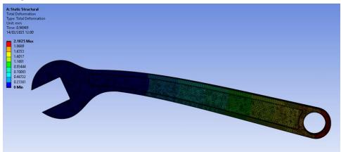
3D model designed and FEA tested in ANSYS space claim – 3D model of a wrench was designed and testing 2 separate materials (Titanium and Steel were chosen for this project), compare the differences between the materials, such as maximum stress & strain, and total deformation. Convergence studies were also performed to achieve the most optimum element size for simulation.
