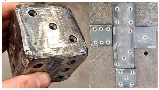
Fabricated a dice and adjustable wrench(not pictured) – within second year of University, a module further developed my fabrication skills. The first project was manufacturing a wrench using a mild steel for the main body and brass for the adjustment wheel. This made use of a fly press to fold a sheet metal plate, to protect the threaded rod as well as create an ergonomic handle comfortable to hold. The second project, the steel die, was to improve MIG welding skills.
