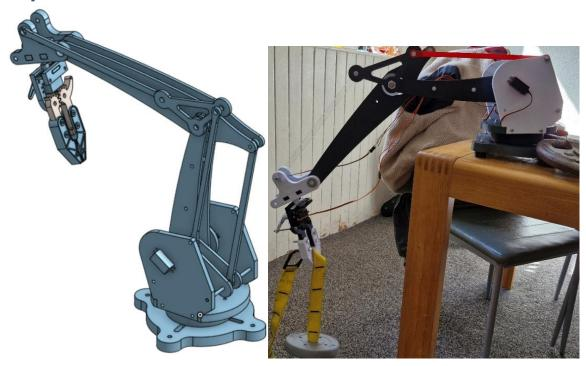
Honours Project with SolidWorks – Designing a lightweight robotic arm capable of carrying a payload of 1kg. Made with 3D printed materials such as ABS and PETG and programmed using an Arduino to allow for closed loop control with the use of an ultrasonic sensor for object detection.
