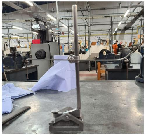
Fabricated a scribe block from bright mild steel – project in college allowed fabrication work with mild steel (milling, drill press, tapping, welding). Some challenges along the way would be the base of the block being poorly cast, having to make use of skills to reinforce.
