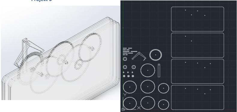
Crude design of a clock for a project and parts using SolidWorks and AutoCAD - Main outcome for skills was designing motion studies within SolidWorks and timings of mechanical linkages for accurate time keeping.
